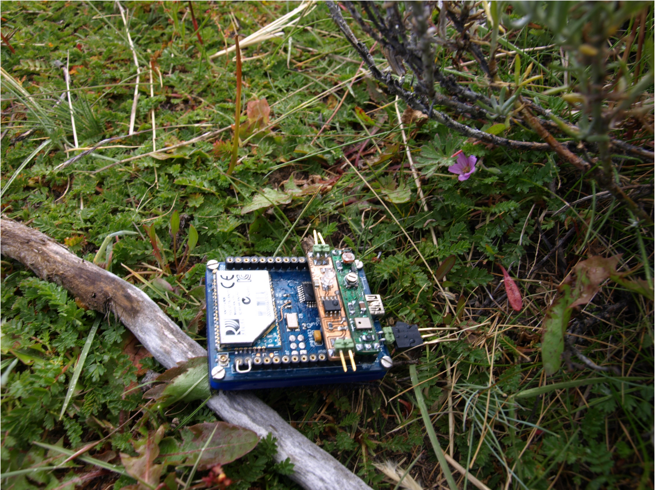
Figure 14 Ukika. Equipment used for detecting ultraviolet, light and temperature detection. Made by artist engineer Martin Hug (2015)
